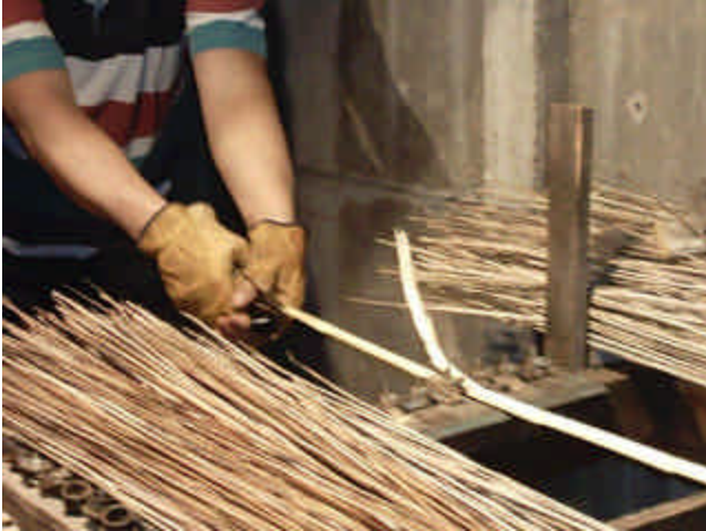
The photo on the left is from Chile, showing a splitting jig.
